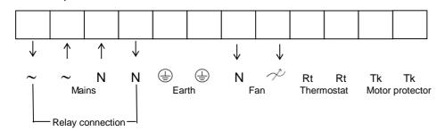
Relay connection: There is always 230V between ~ and N when the transformer knob is in one of the positions 1-5. If the motor protection is not in use, Tk shall be looped together.
